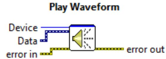
Plays data from the sound output device using finite sampling. This Express VI automatically configures an output task and clears the task after the output completes.
